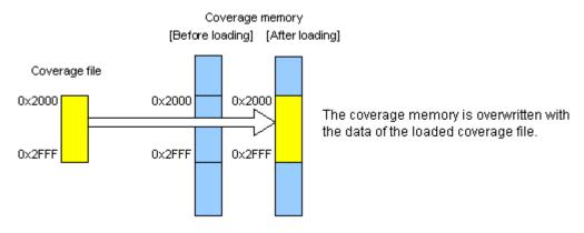
Figure 5.99 Schematic of load modes when selecting overwrite
